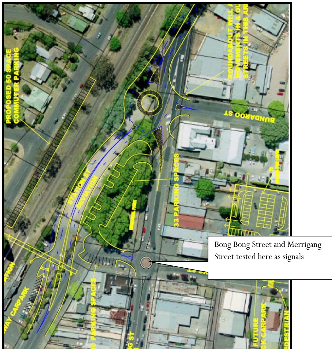
Figure 7-2 – Preliminary layout of proposed reconfiguration of the intersection of Station Street, Bong Bong Street and Bundaroo Street as a two-lane roundabout
