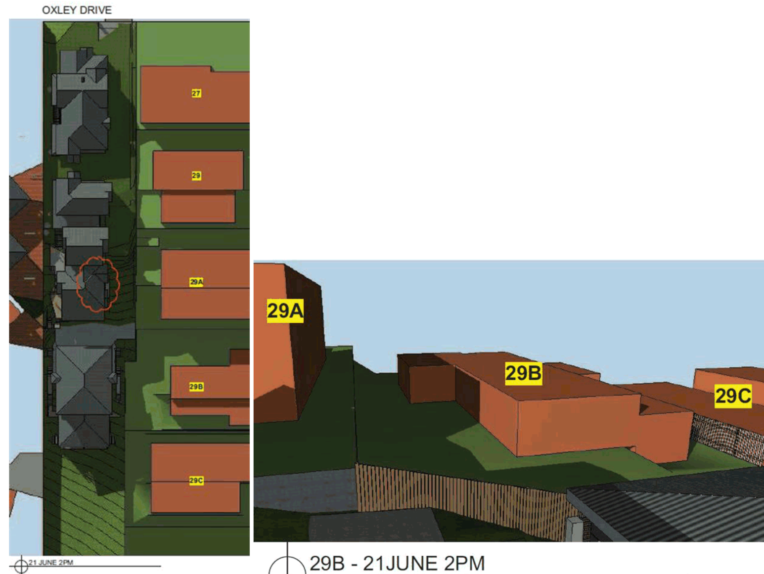
2:00 pm 21 June - Shadow impact upon 29B Oxley Drive cast from 29 A Oxley Drive and proposed development does not affect solar access to western facing living room window of 29B Oxley Drive.
