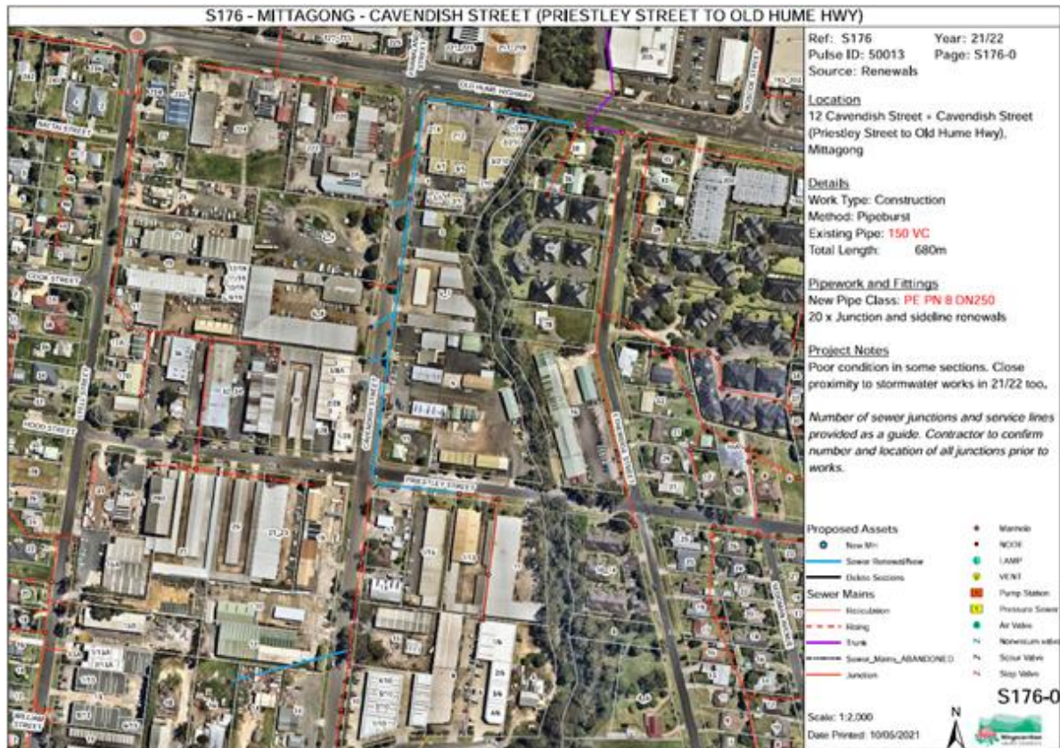
Figure 2. Overview of the S176 – Mittagong – Cavendish Street section for upsizing and renewal.
