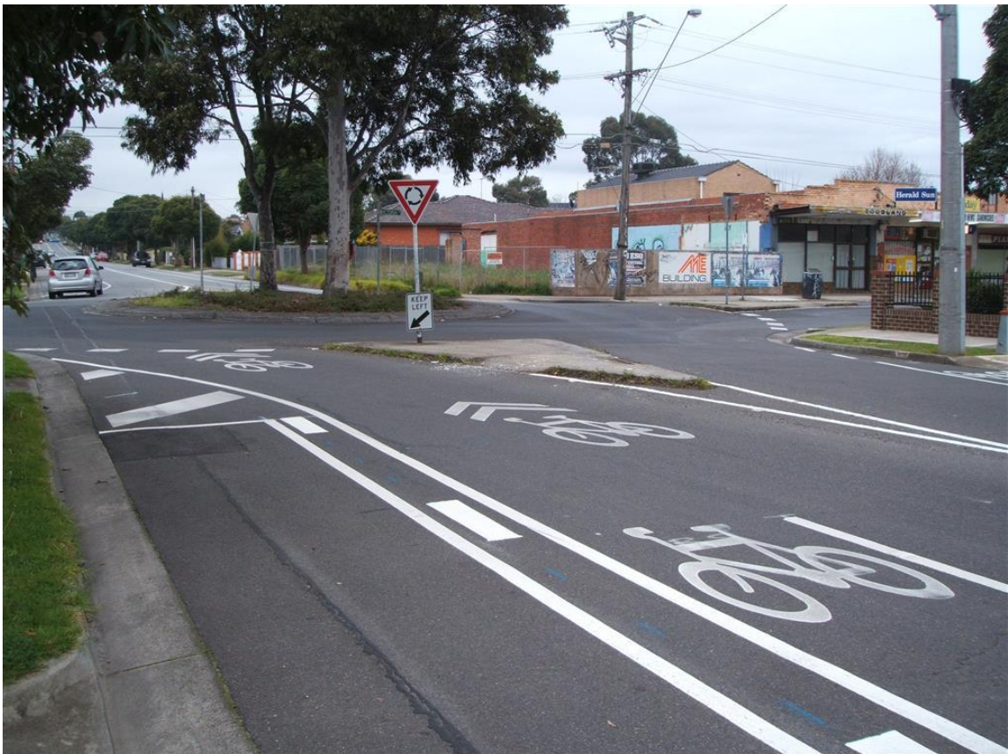
Figure 5.20: Sharrow Road Markings – Raglan Street, Preston, Victoria
