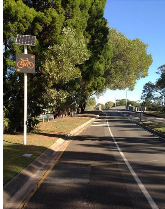
Figure 5.15: Bicycle activated warning sign – Noosa Parade, Noosa, Queensland
