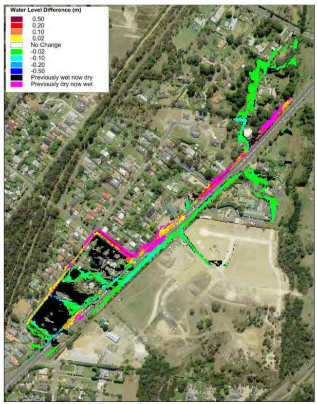
Plate 29 20% AEP Flood Level Difference Map for FM7
