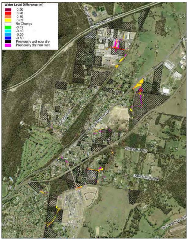
Plate 4 Flood Level Difference Map for the 20% AEP future catchment development scenario
