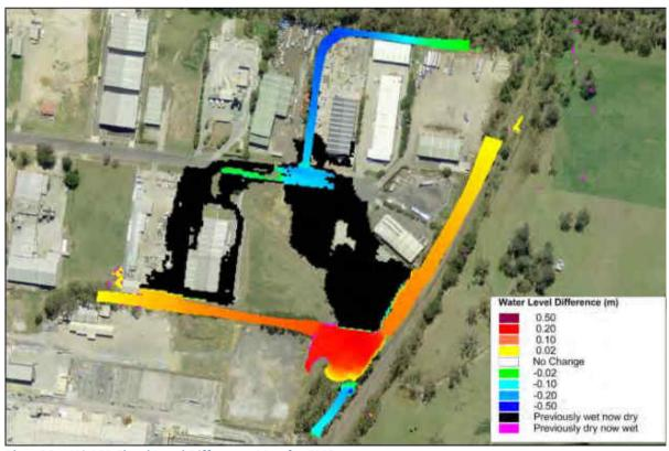
Plate 36 1% AEP Flood Level Difference Map for FM9
