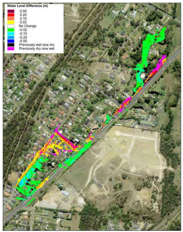
Plate 30 1% AEP Flood Level Difference Map for FM7
