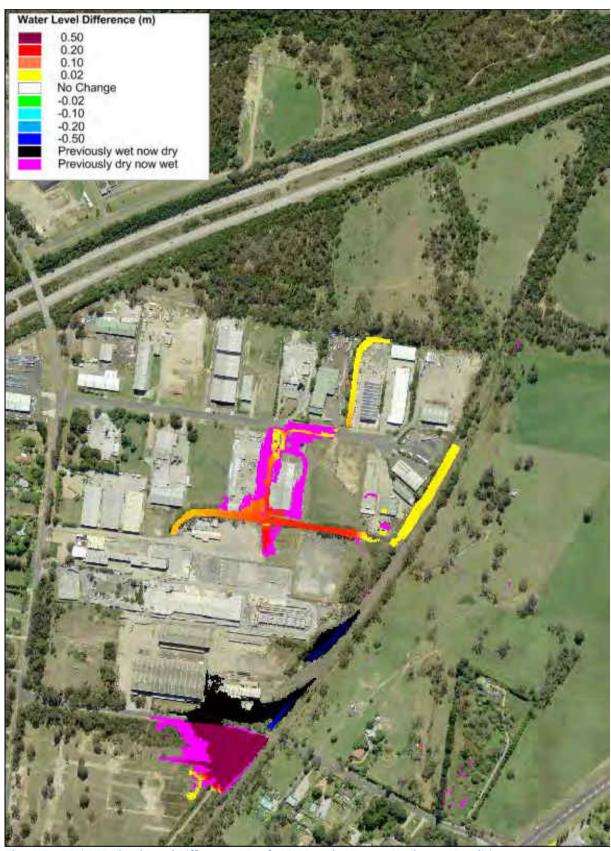
Plate 17 20% AEP Flood Level Difference Map for FM2 under Future Catchment Conditions
