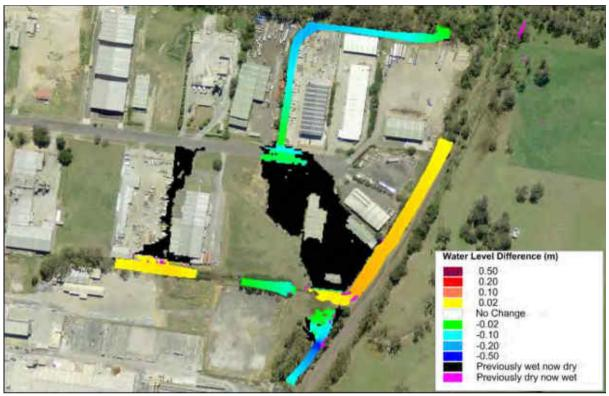
Plate 35 20% AEP Flood Level Difference Map for FM9
