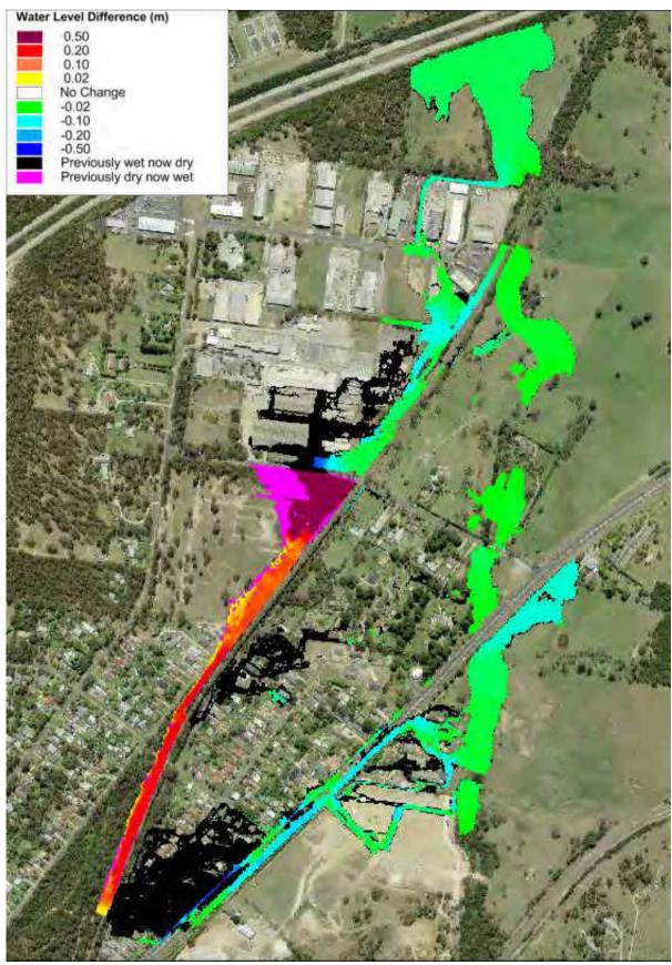
Plate 32 1% AEP Flood Level Difference Map for FM8
