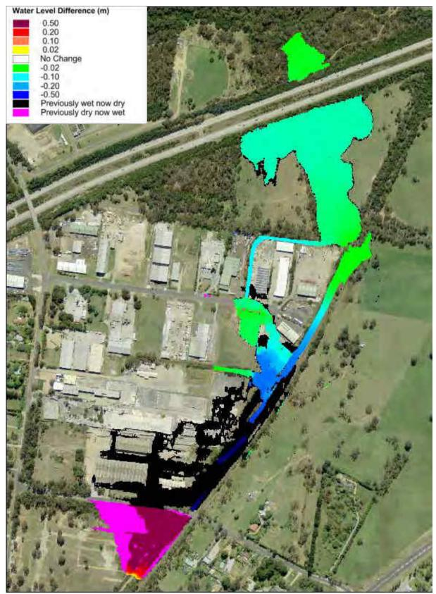
Plate 16 1% AEP Flood Level Difference Map for FM2
