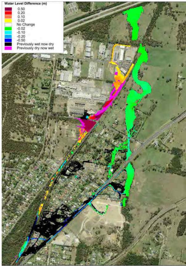
Plate 39 20% AEP Flood Level Difference Map for FM10
