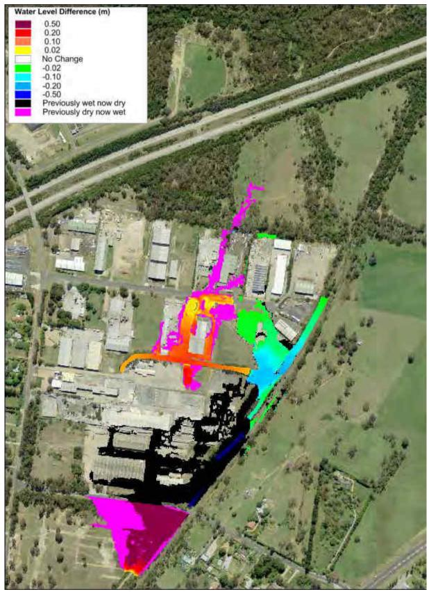
Plate 18 1% AEP Flood Level Difference Map for FM2 under Future Catchment Conditions
