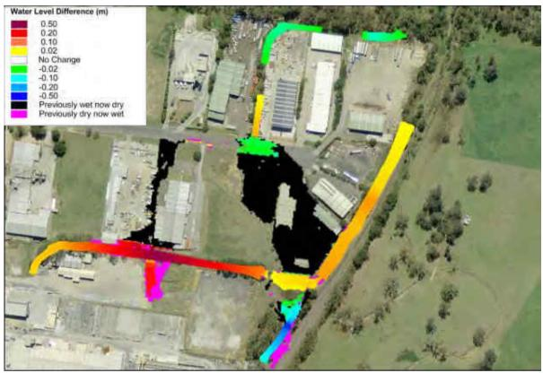
Plate 37 20% AEP Flood Level Difference Map for FM9 under Future Catchment Conditions
