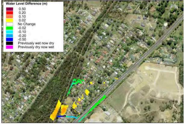
Plate 28 1% AEP Flood Level Difference Map for FM6
