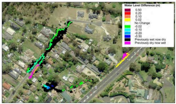
Plate 25 20% AEP Flood Level Difference Map for FM5
