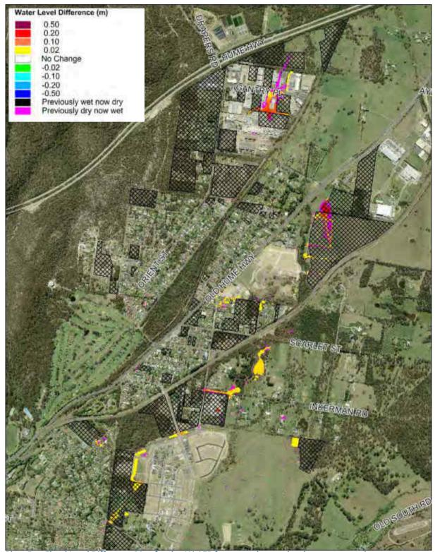
Plate 5 Flood Level Difference Map for the 1% AEP future catchment development scenario
