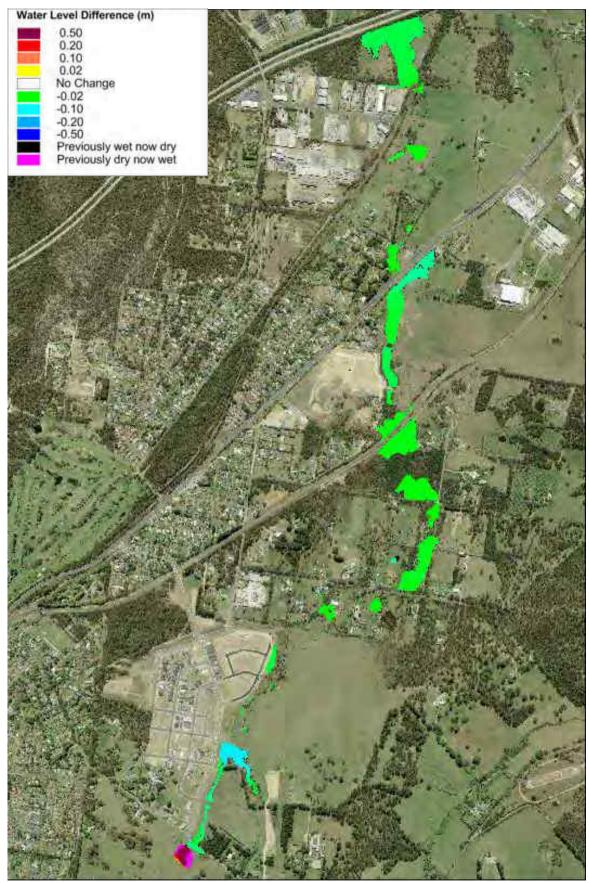
Plate 20 1% AEP Flood Level Difference Map for FM3
