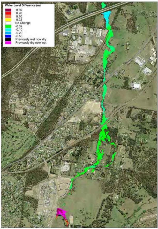
Plate 13 20% AEP Flood Level Difference Map for Oldfield Road Basin Modifications (FM1)
