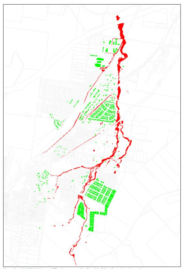
Plate 49 1% AEP high hazard/floodway areas (red) and building footprints (green)
