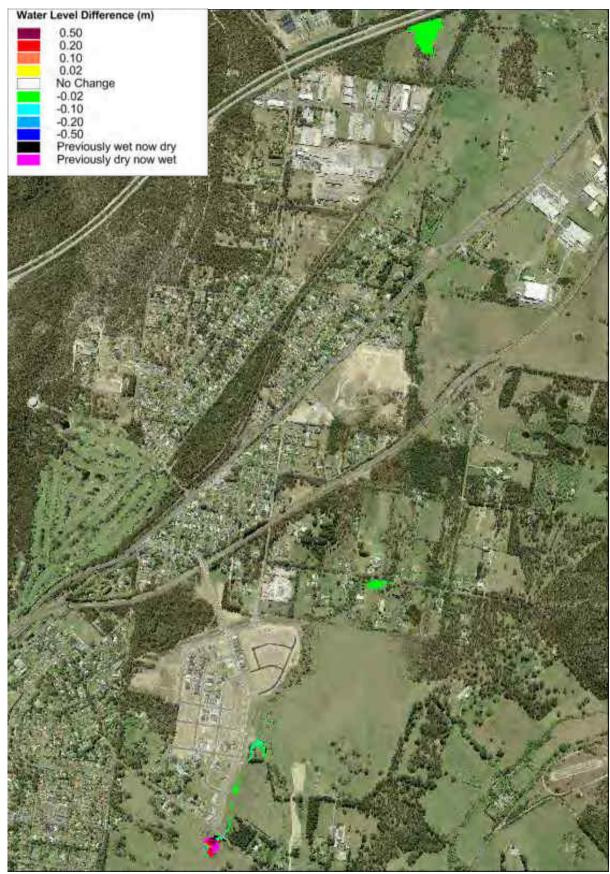
Plate 19 20% AEP Flood Level Difference Map for FM3
