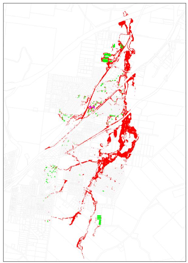
Plate 48 1% AEP low hazard areas (red) and buildings subject to frequent above floor inundation (green)
