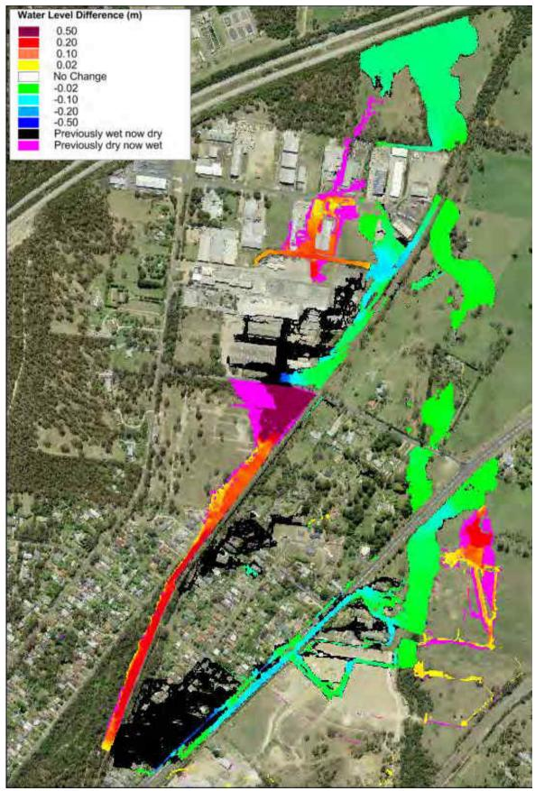
Plate 34 1% AEP Flood Level Difference Map for FM8 under Future Catchment Conditions
