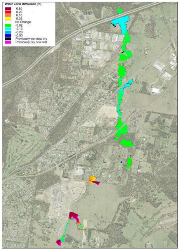
Plate 24 1% AEP Flood Level Difference Map for FM1, FM3 & FM4
