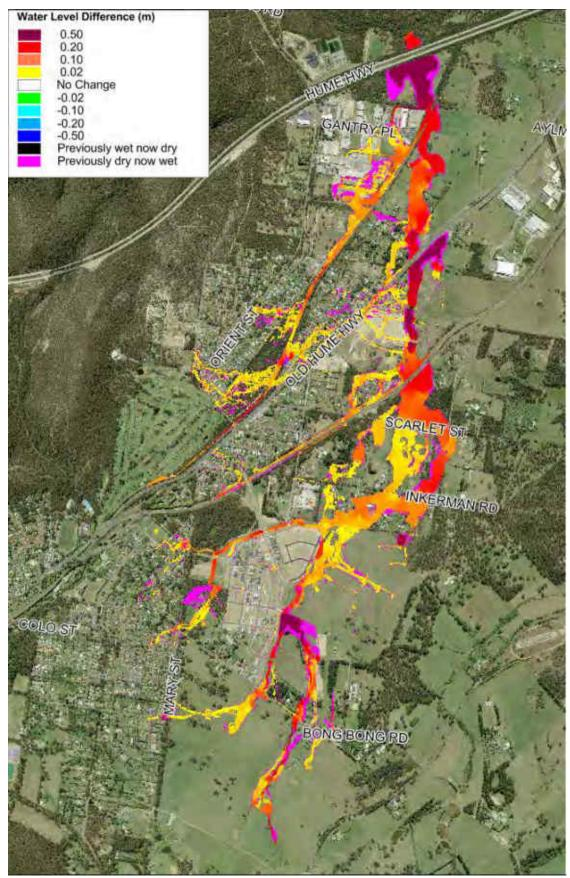
Plate 9 Flood level difference map for 0.2%AEP against 1%AEP
