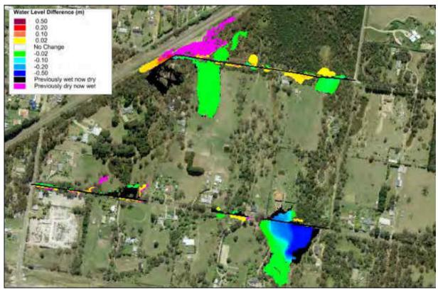
Plate 53 1% AEP Flood Level Difference Map for RM7
