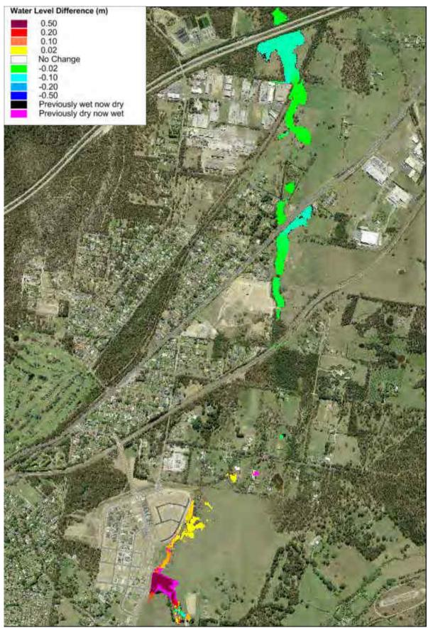
Plate 14 1% AEP Flood Level Difference Map for Oldfield Road Basin Modifications (FM1)
