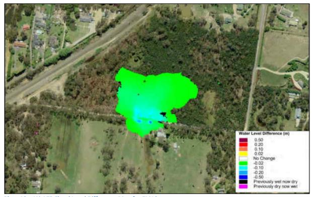
Plate 46 1% AEP Flood Level Difference Map for FM13
