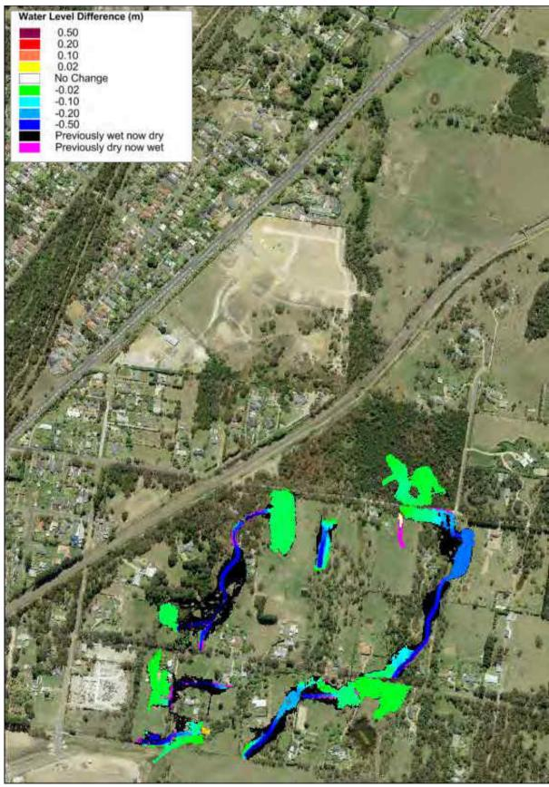
Plate 43 20% AEP Flood Level Difference Map for FM12
