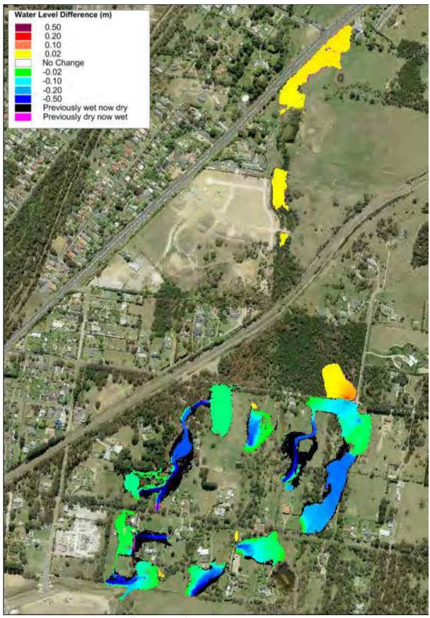
Plate 44 1% AEP Flood Level Difference Map for FM12
