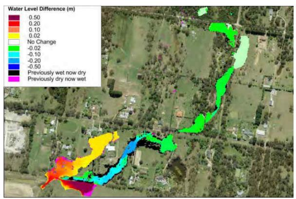
Plate 21 20% AEP Flood Level Difference Map for FM4
