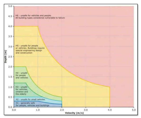
Plate 2 Flood Hazard Vulnerability Curves (AIDR, 2014)
