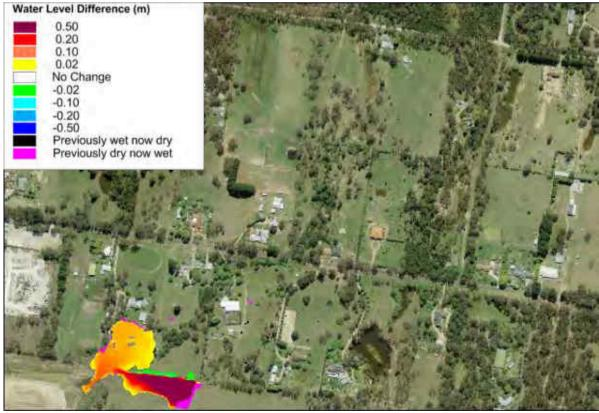
Plate 22 1% AEP Flood Level Difference Map for FM4
