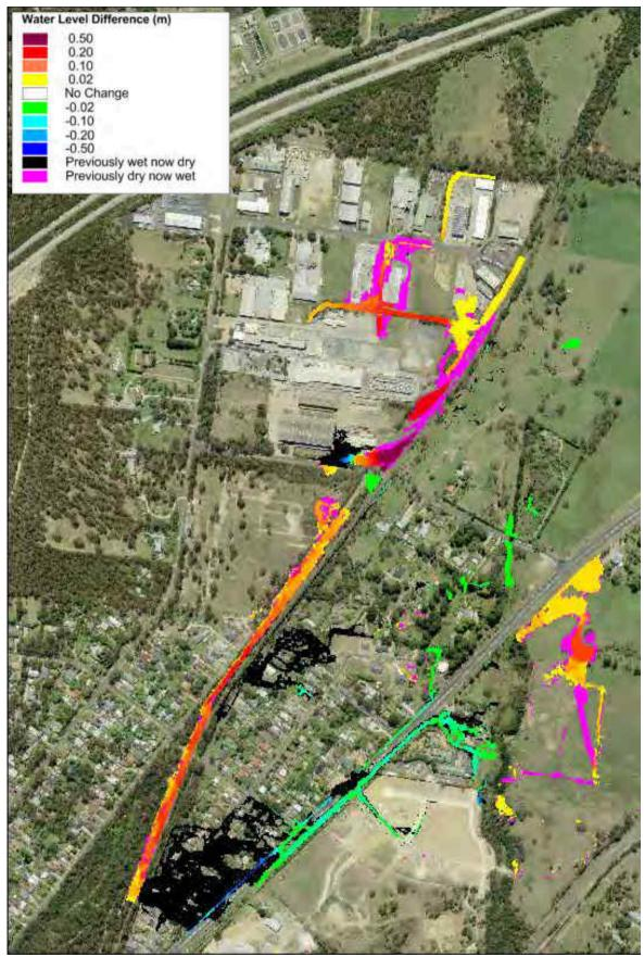
Plate 33 20% AEP Flood Level Difference Map for FM8 under Future Catchment Conditions
