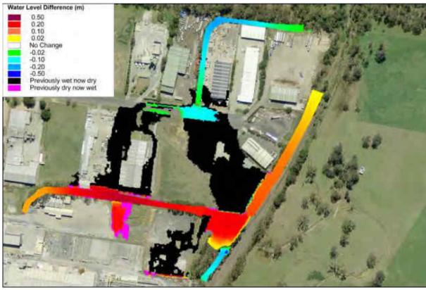
Plate 38 1% AEP Flood Level Difference Map for FM9 under Future Catchment Conditions
