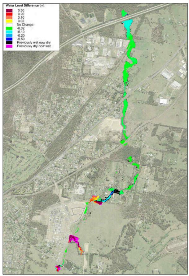
Plate 23 20% AEP Flood Level Difference Map for FM1, FM3 & FM4
