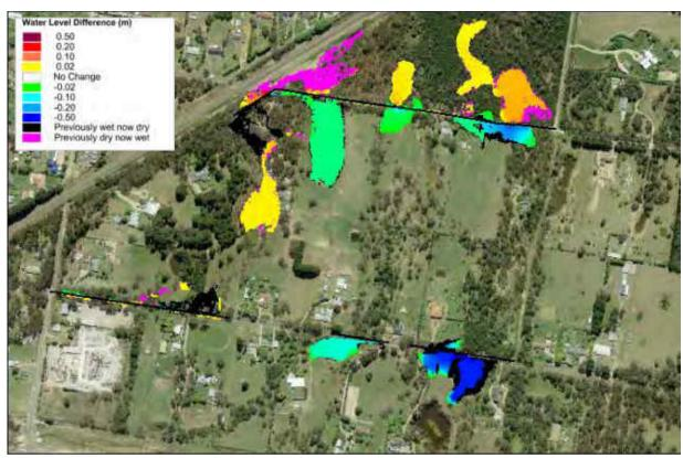
Plate 52 20% AEP Flood Level Difference Map for RM7
