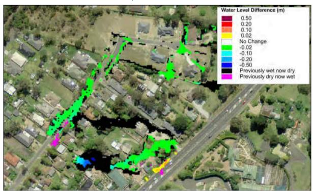
Plate 26 1% AEP Flood Level Difference Map for FM5
