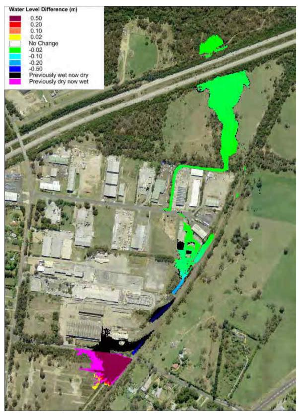
Plate 15 20% AEP Flood Level Difference Map for FM2
