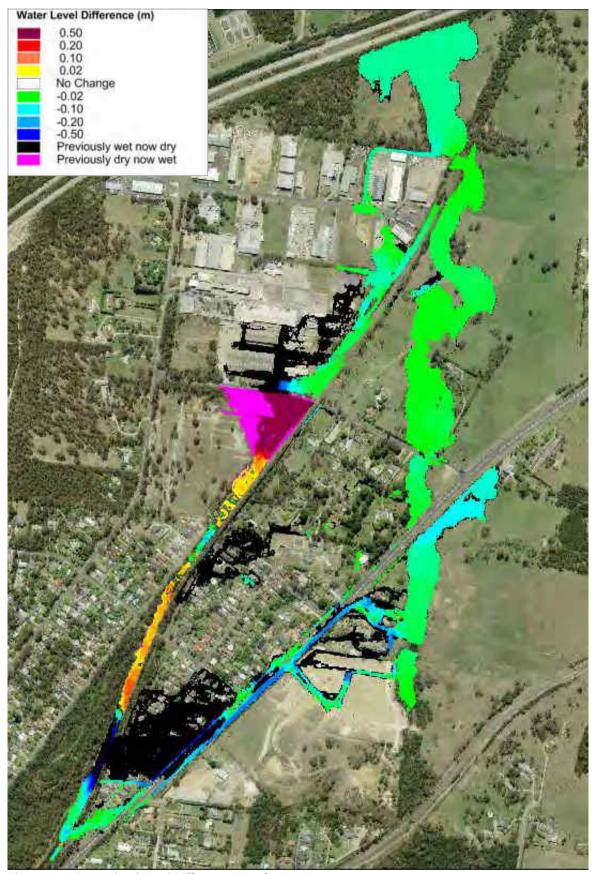
Plate 40 1% AEP Flood Level Difference Map for FM10
