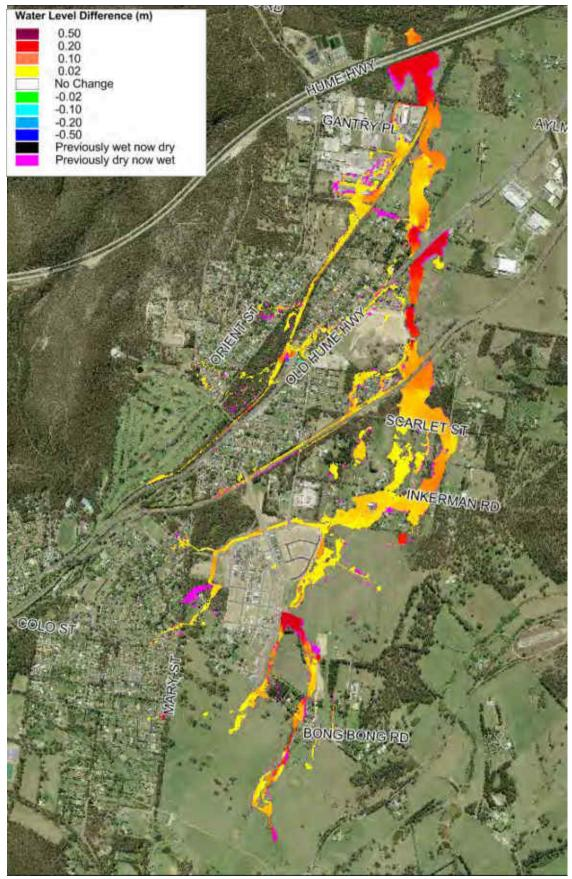
Plate 8 Flood level difference map for 0.5%AEP against 1%AEP
