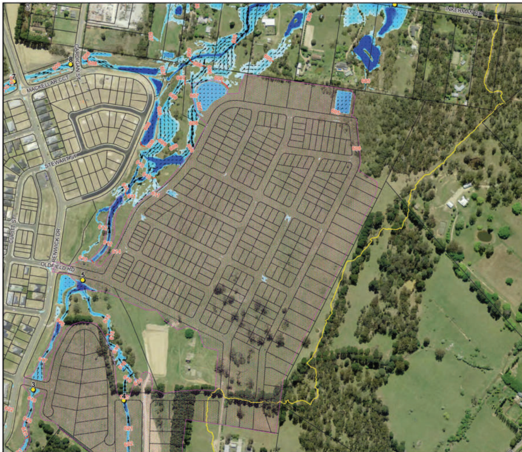
Figure 4.3: Floodwater Depths, Levels and Velocities for the 20% AEP Flood
