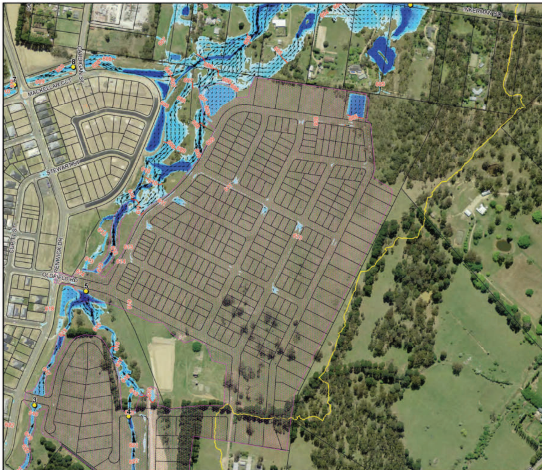
Figure 6.3: Floodwater Depths, Levels and Velocities for the 5% AEP Flood
