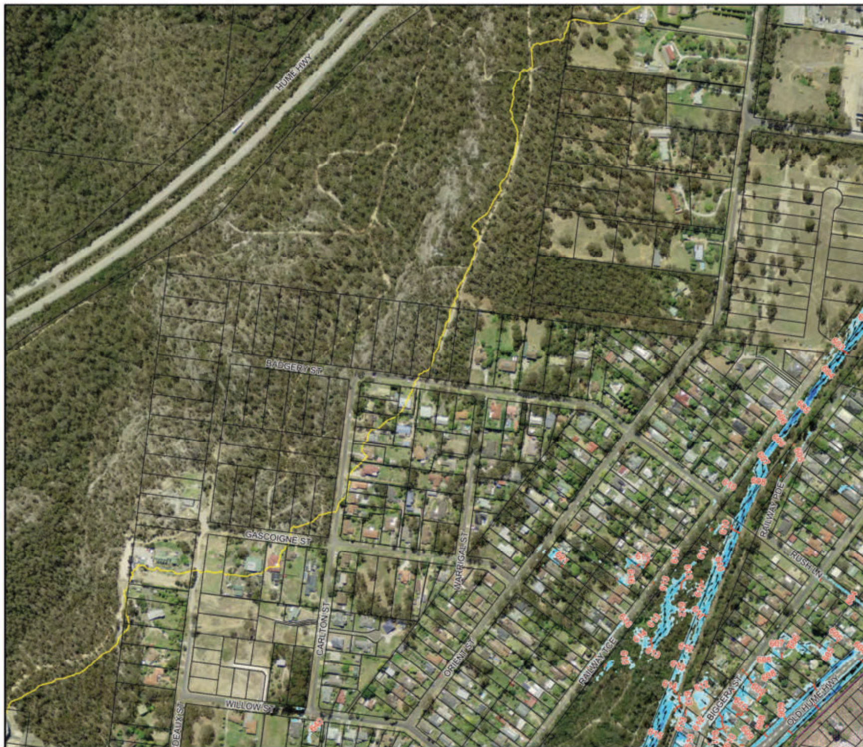
Figure 8.6: Floodwater Depths, Levels and Velocities for the 1% AEP Flood
