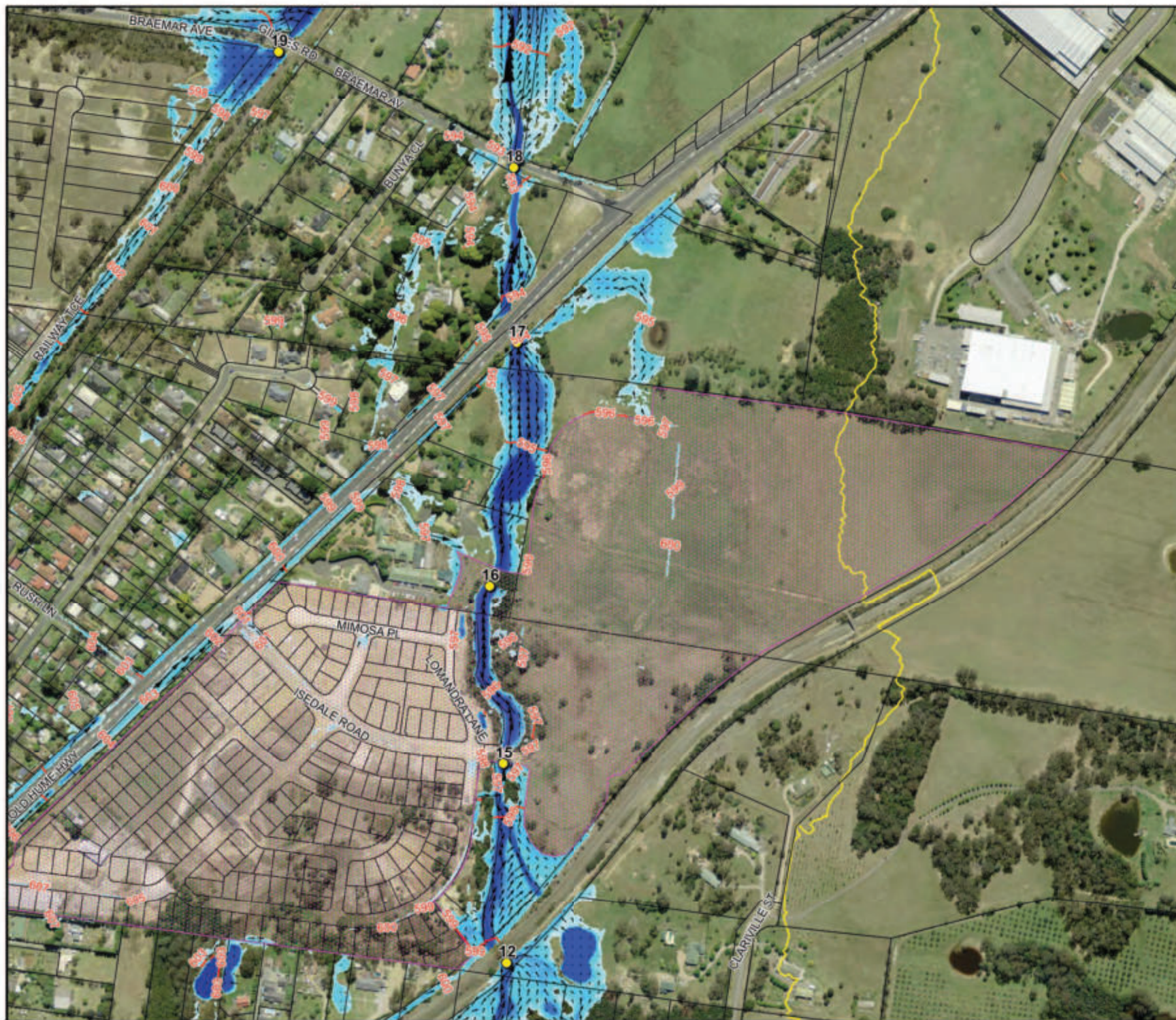
Figure 5.7: Floodwater Depths, Levels and Velocities for the 10% AEP Flood
