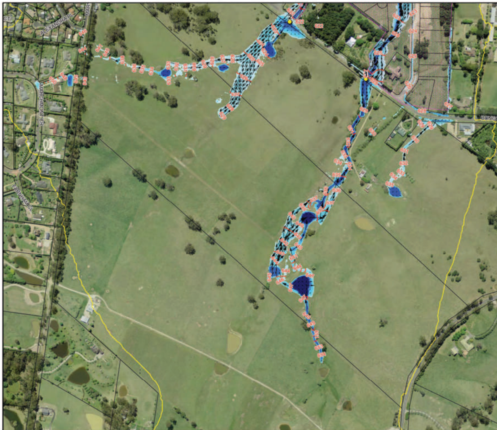
Figure 10.1: Floodwater Depths, Levels and Velocities for the 0.2% AEP Flood
