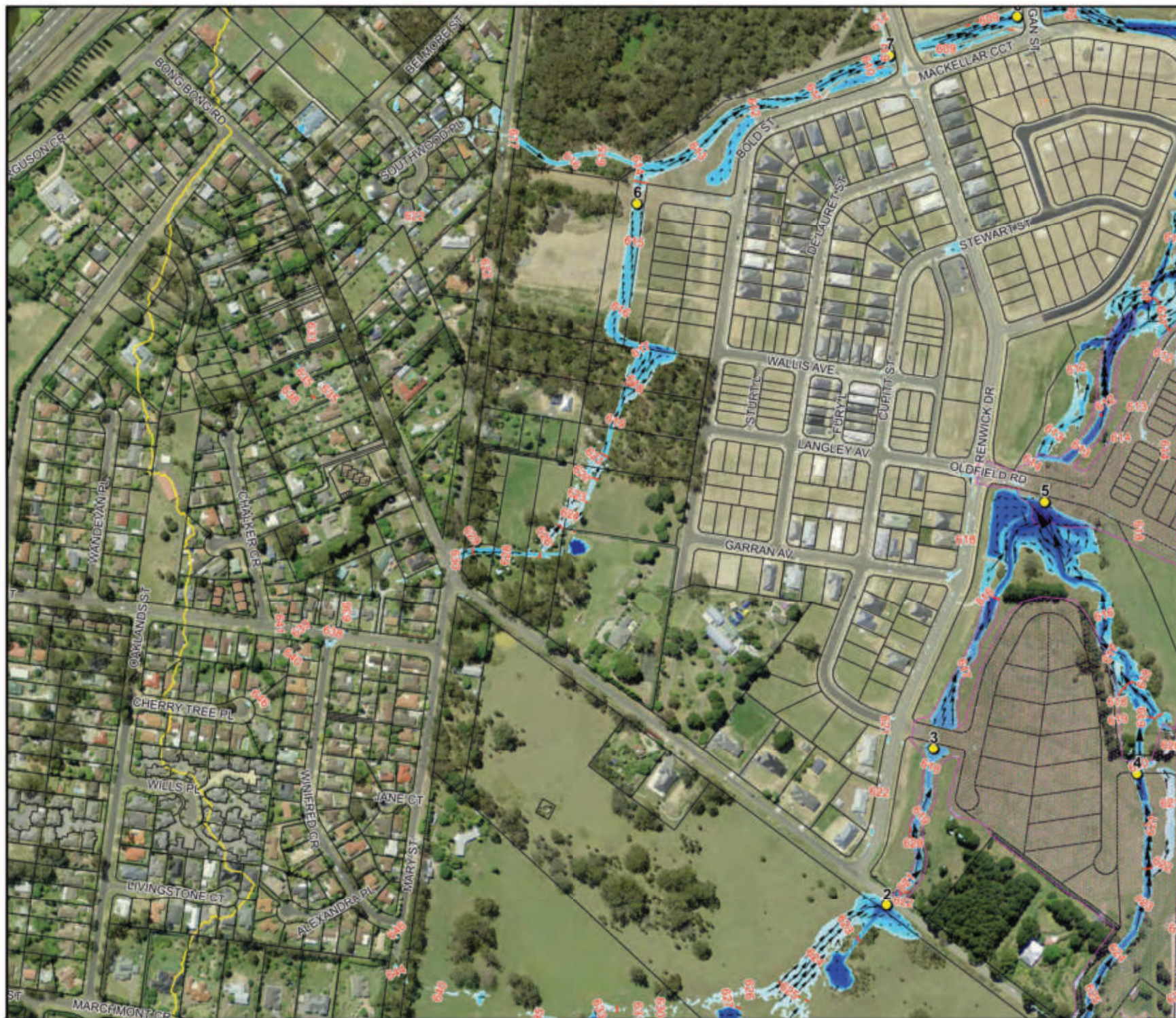
Figure 7.2: Floodwater Depths, Levels and Velocities for the 2% AEP Flood
