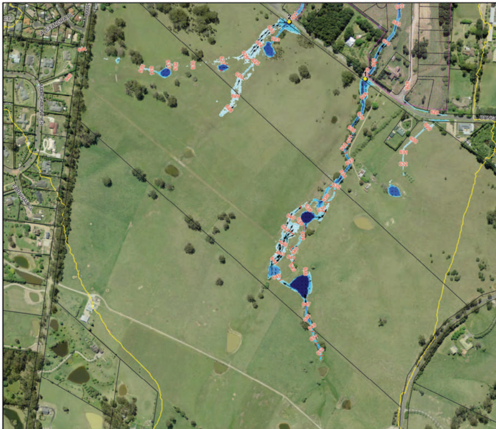
Figure 6.1: Floodwater Depths, Levels and Velocities for the 5% AEP Flood
