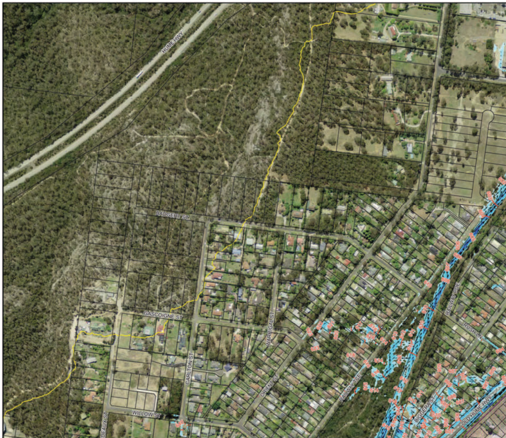
Figure 10.6: Floodwater Depths, Levels and Velocities for the 0.2% AEP Flood
