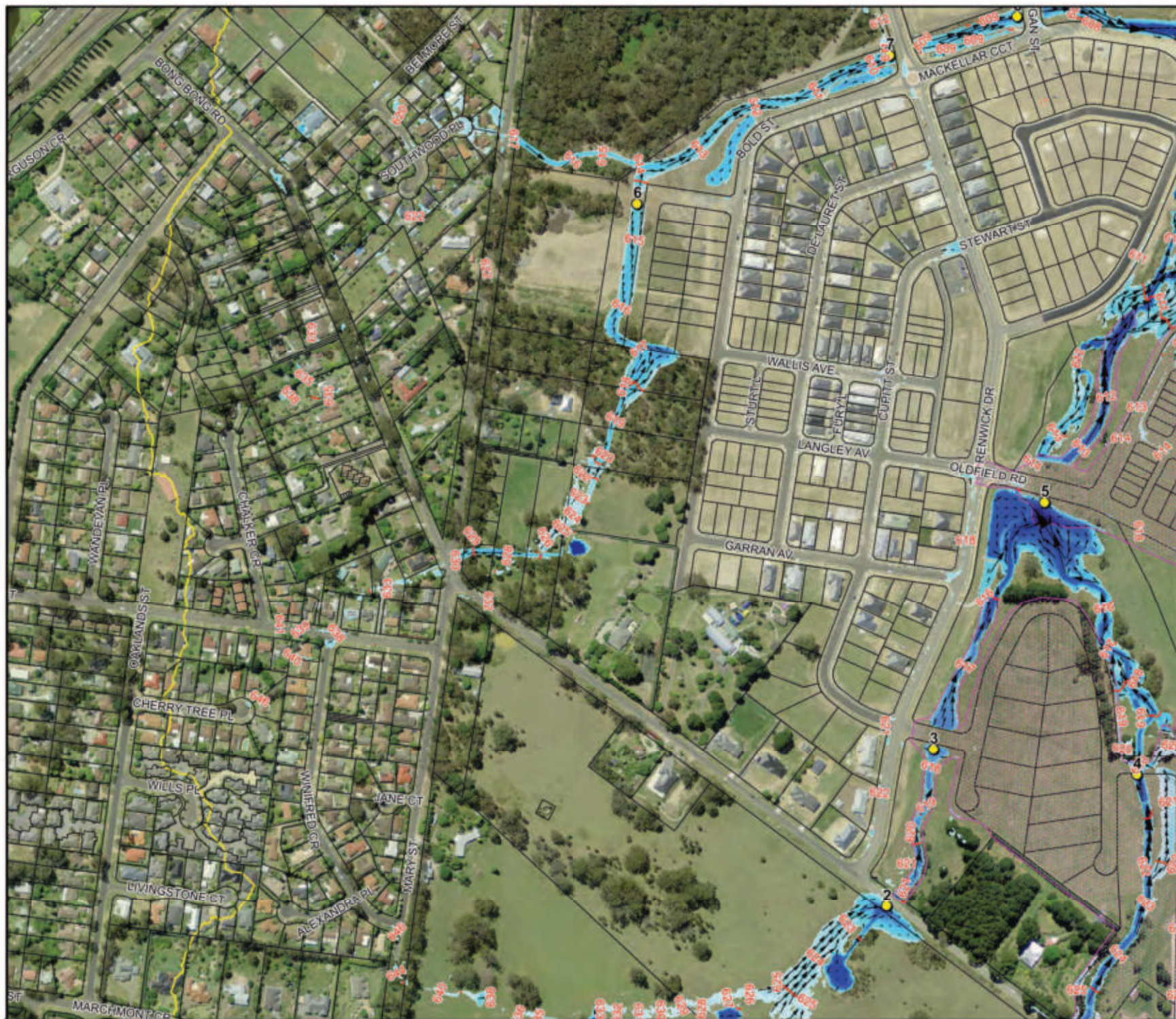
Figure 8.2: Floodwater Depths, Levels and Velocities for the 1% AEP Flood
