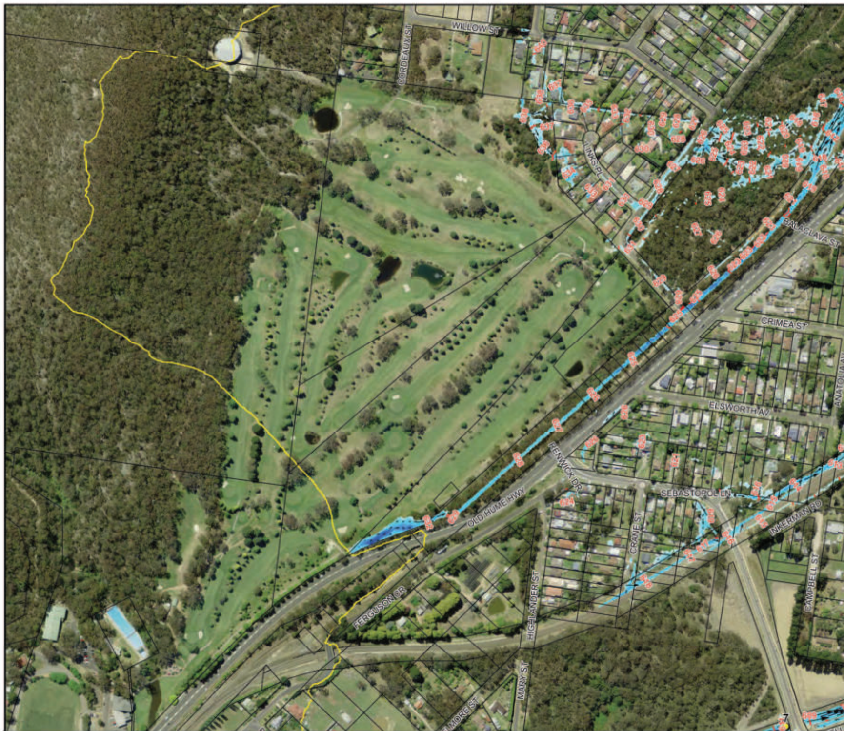
Figure 9.4: Floodwater Depths, Levels and Velocities for the 0.5% AEP Flood
