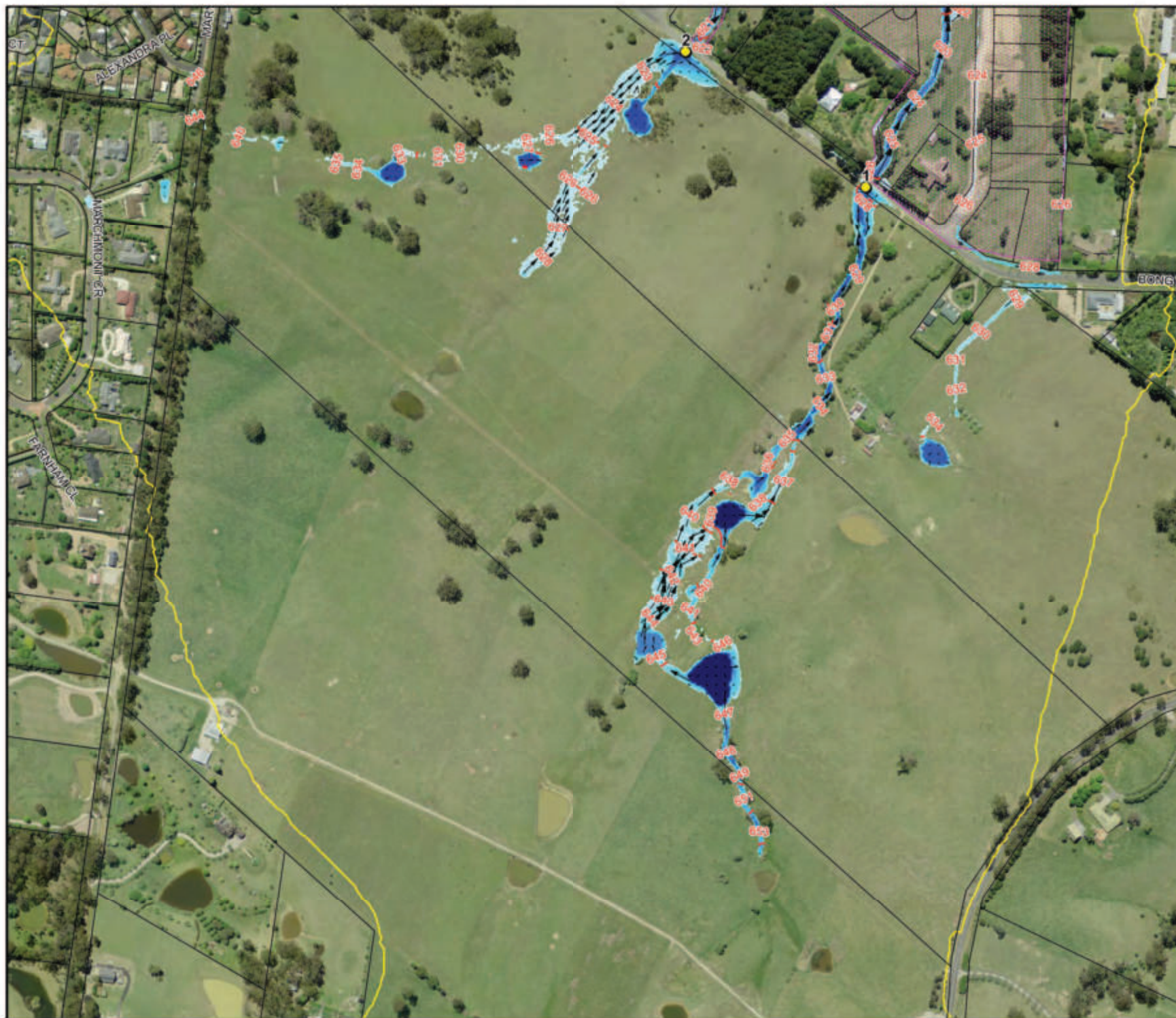
Figure 7.1: Floodwater Depths, Levels and Velocities for the 2% AEP Flood
