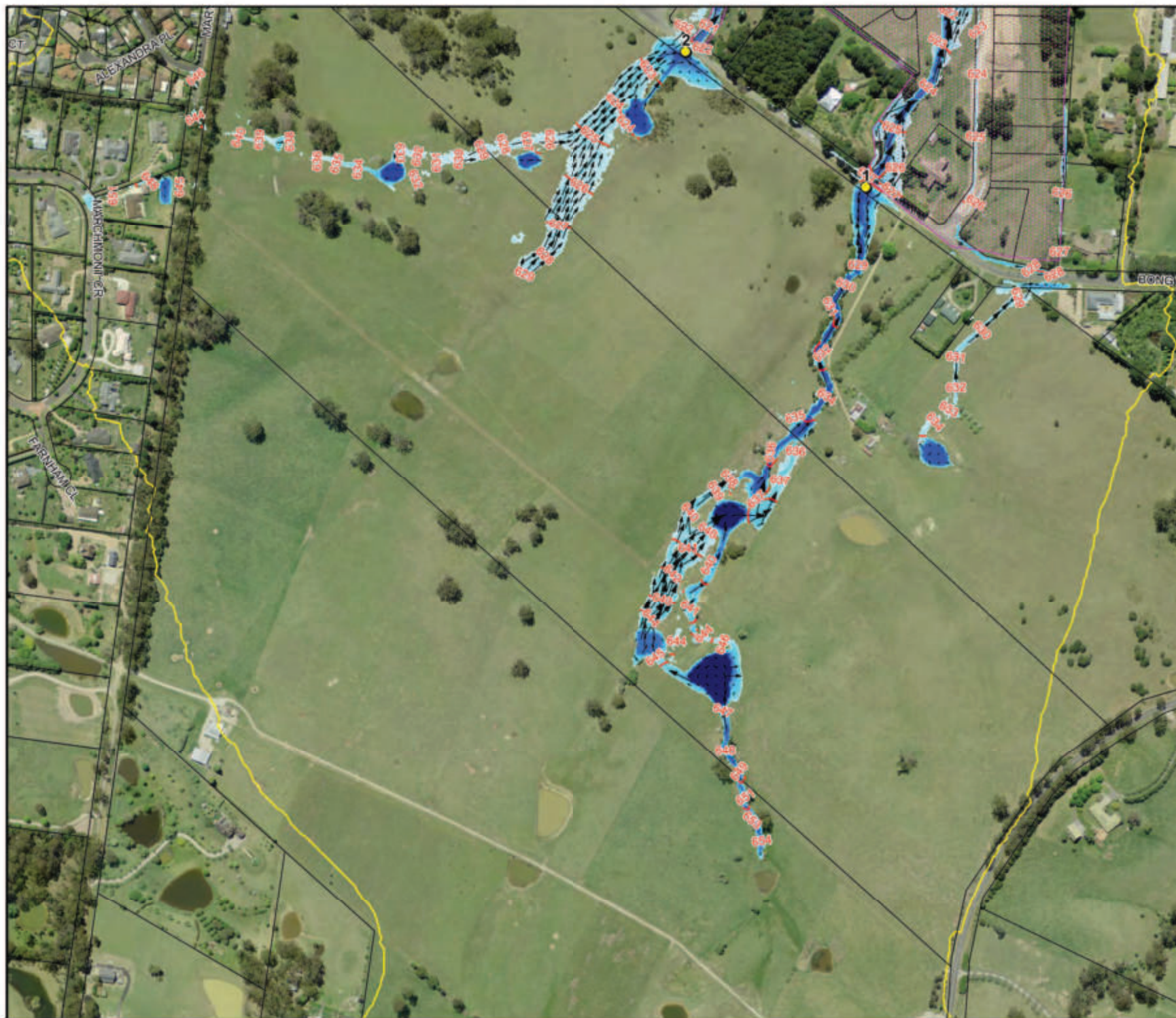
Figure 9.1: Floodwater Depths, Levels and Velocities for the 0.5% AEP Flood
