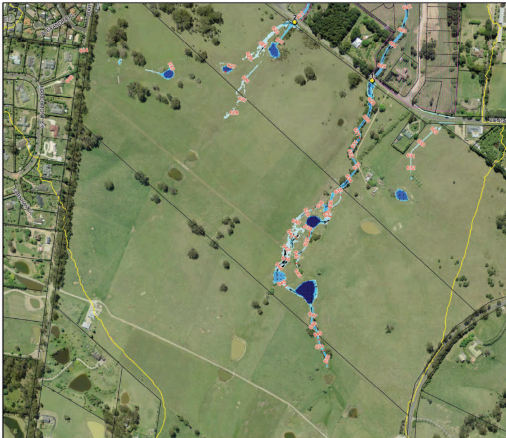
Figure 4.1: Floodwater Depths, Levels and Velocities for the 20% AEP Flood
