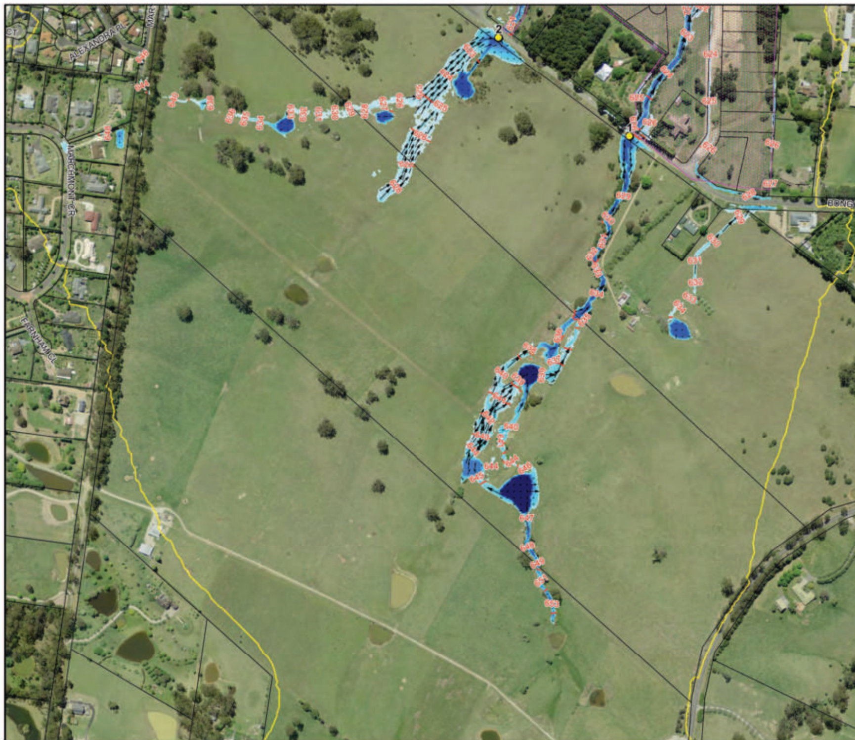
Figure 8.1: Floodwater Depths, Levels and Velocities for the 1% AEP Flood
