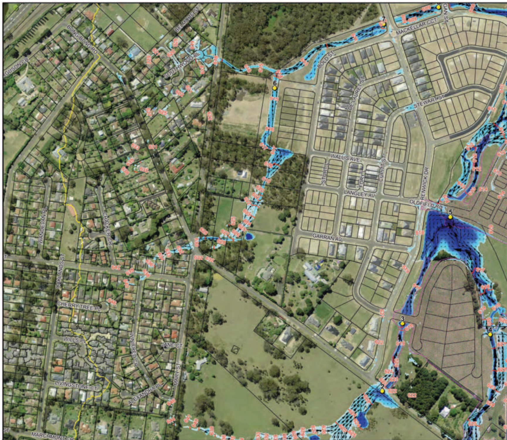
Figure 10.2: Floodwater Depths, Levels and Velocities for the 0.2% AEP Flood
