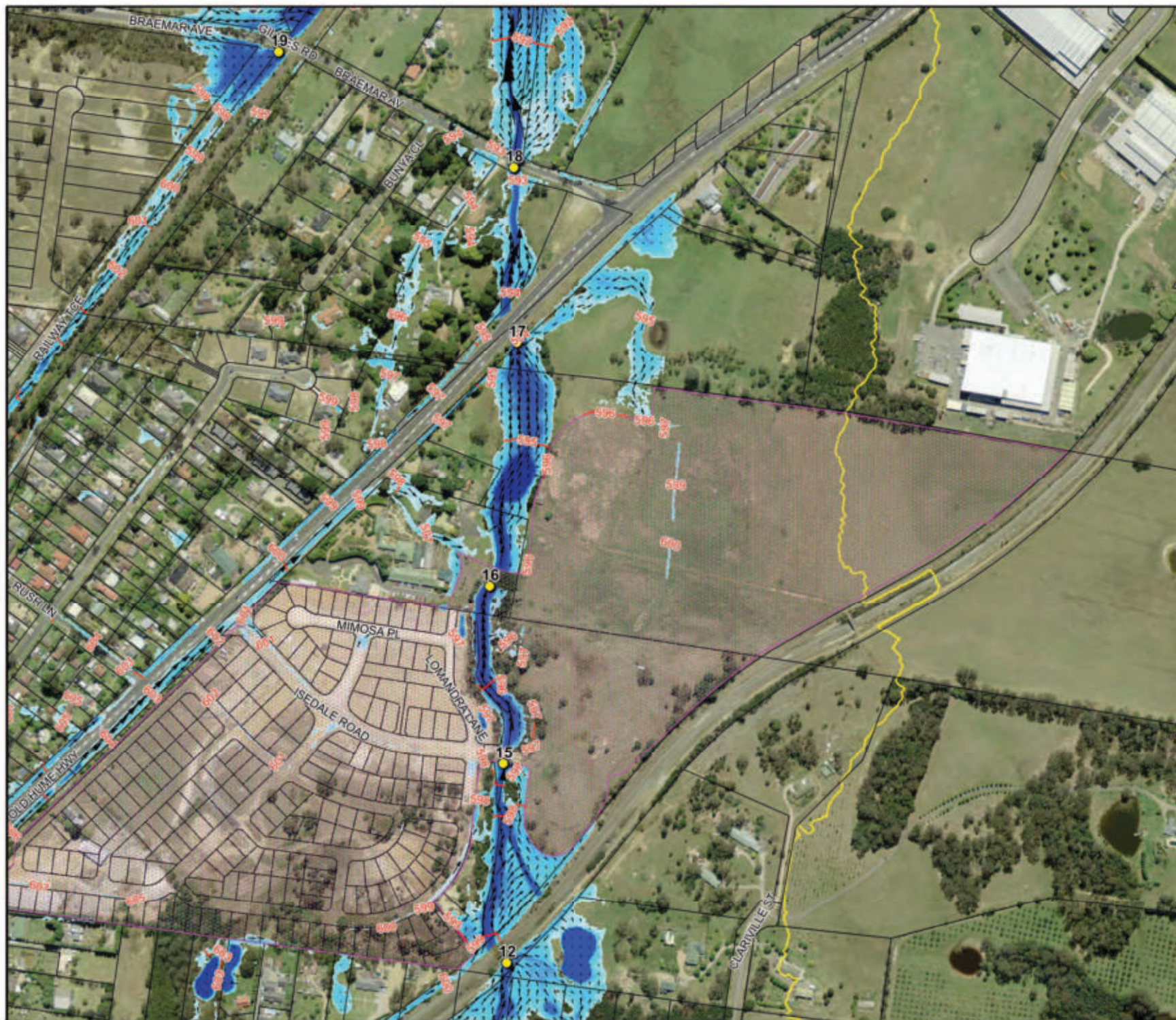
Figure 6.7: Floodwater Depths, Levels and Velocities for the 5% AEP Flood
