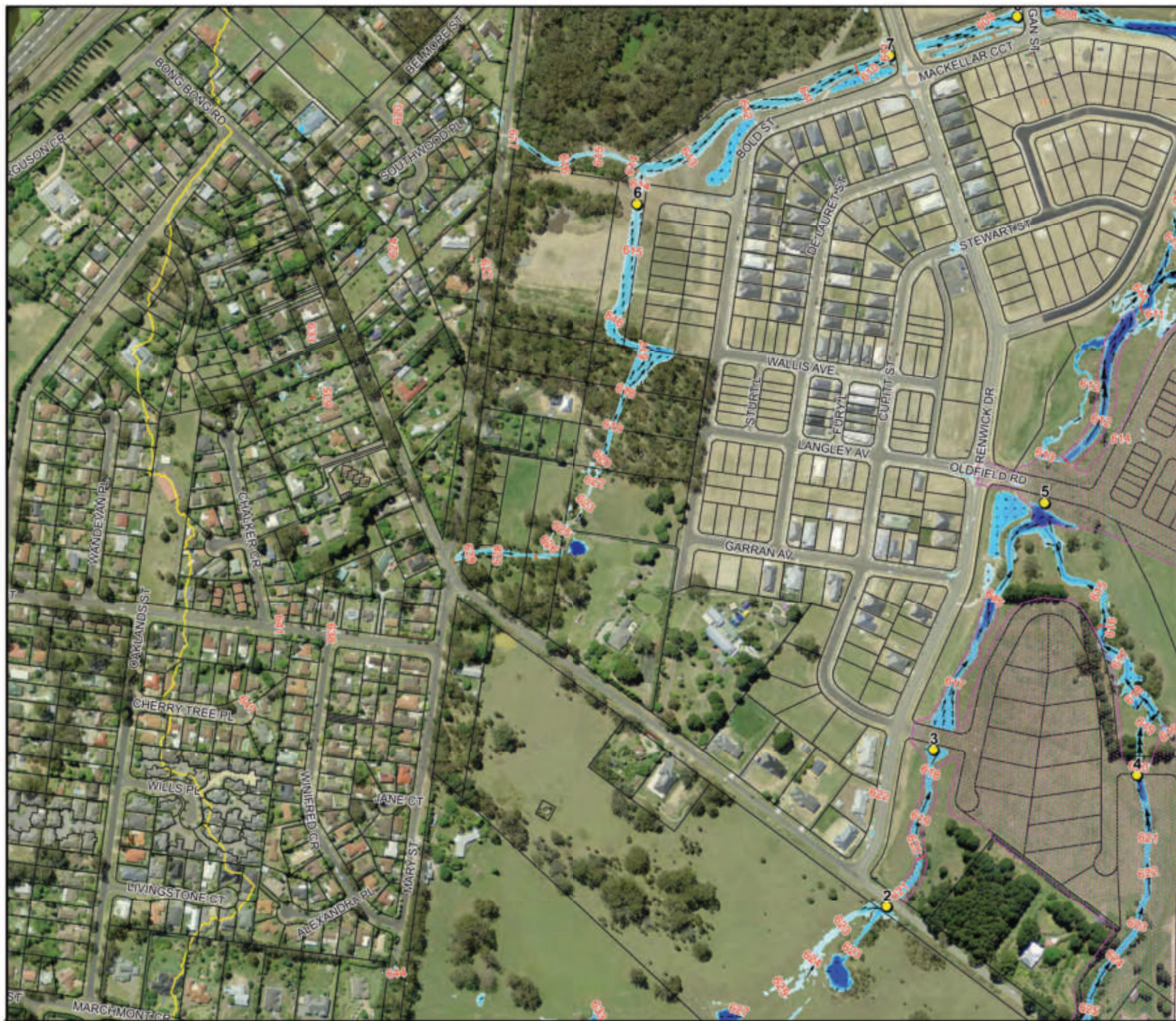
Figure 4.2: Floodwater Depths, Levels and Velocities for the 20% AEP Flood
