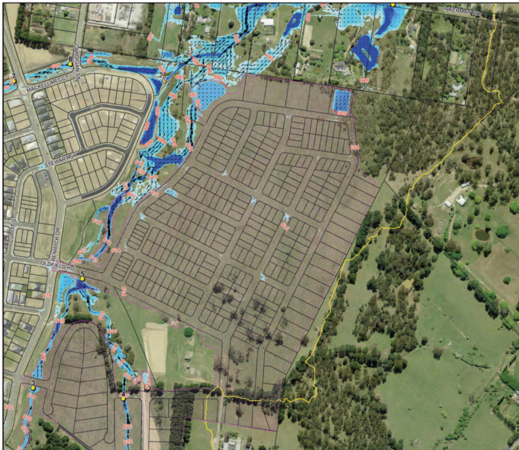
Figure 5.3: Floodwater Depths, Levels and Velocities for the 10% AEP Flood
