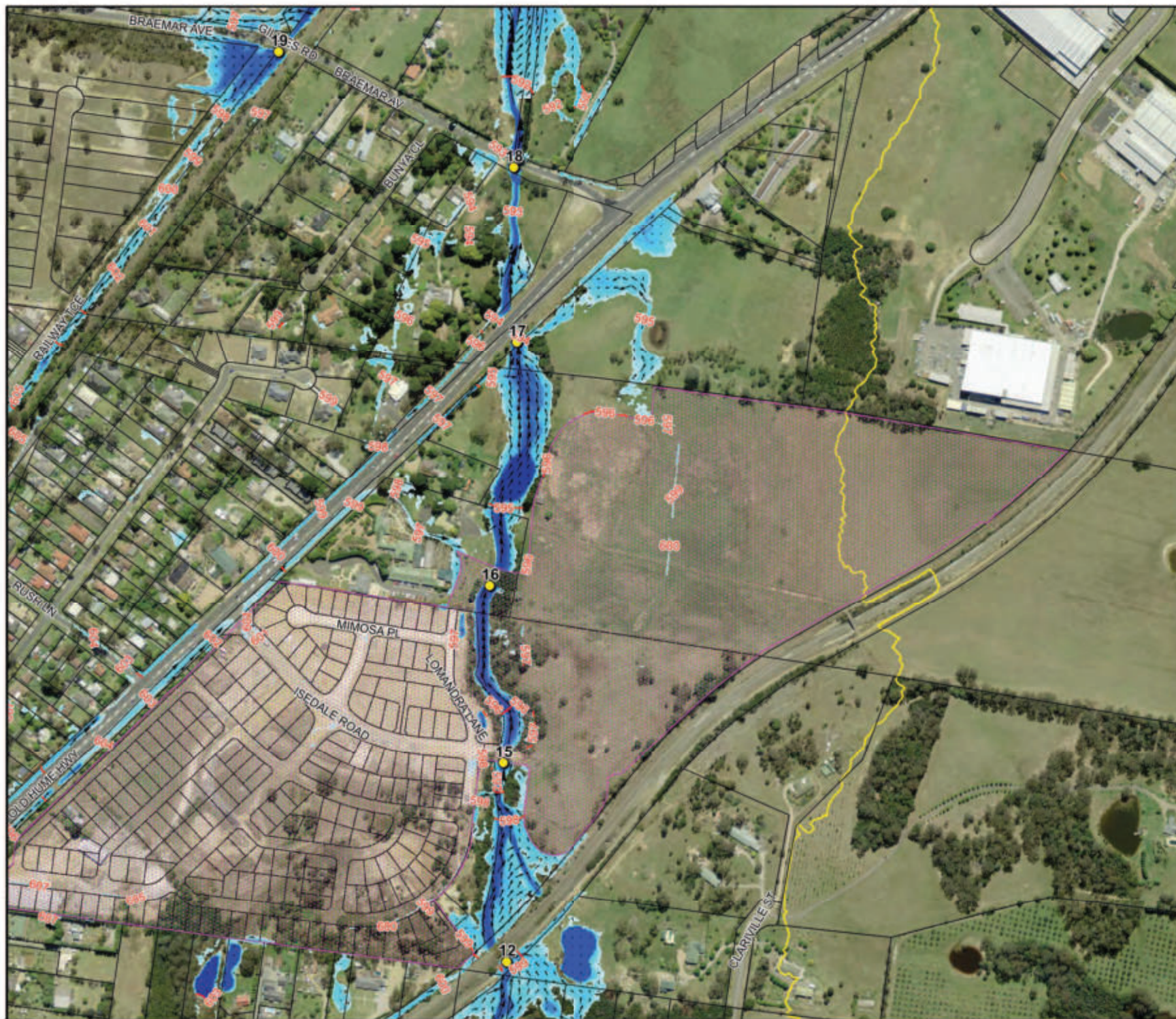
Figure 4.7: Floodwater Depths, Levels and Velocities for the 20% AEP Flood
