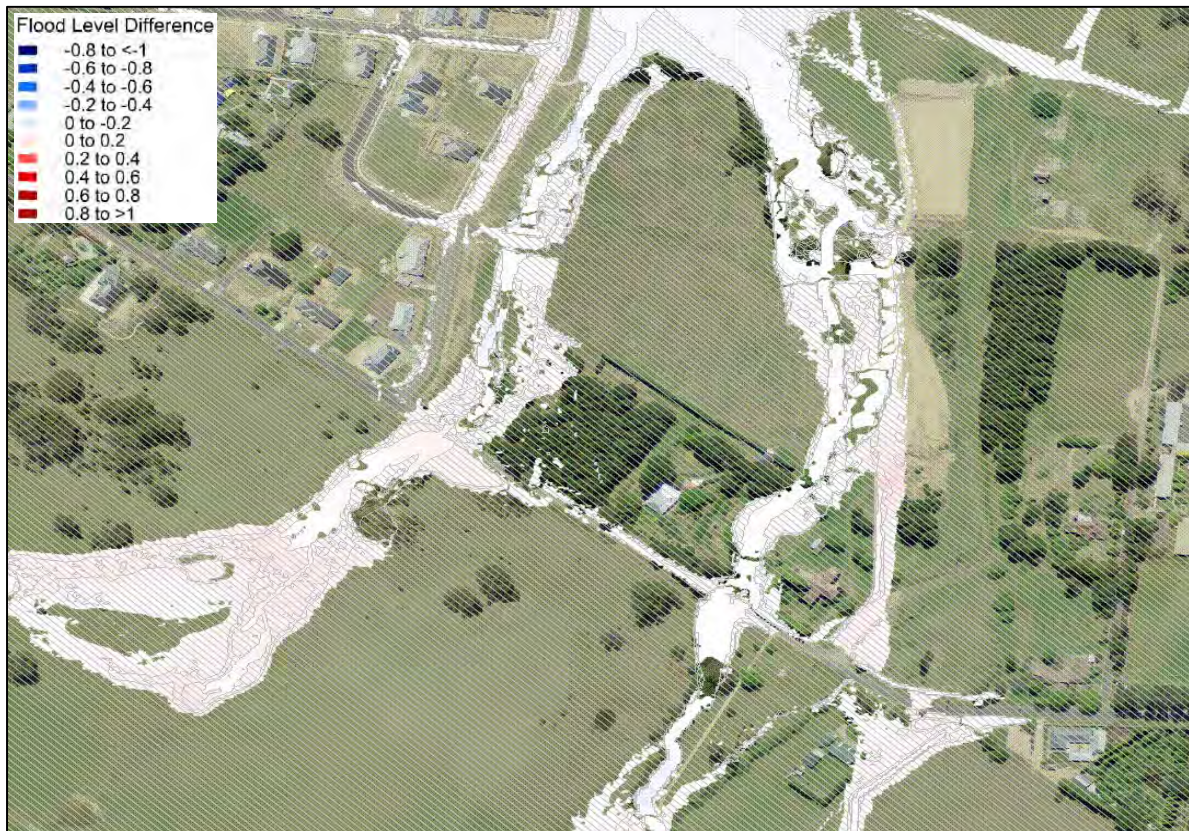
Plate 20 Predicted Change in Peak 1% AEP Flood Levels with increase in Manning's 'n' across flood storage/fringe areas (hatched) in the upper area of the Renwick development
