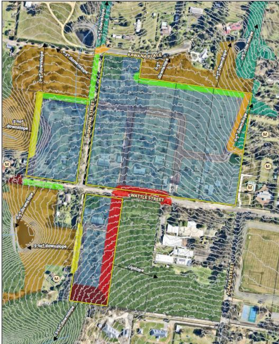
Figure 6 Bushfire Hazard Analysis and Asset Protection Zone
