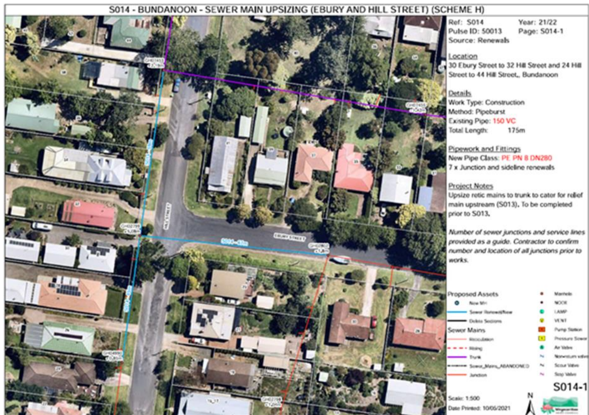
Figure 1. Overview of the S014 - Bundanoon (Ebury Street and Hill Street) section for upsizing.
