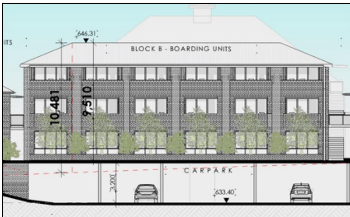
Figure 5: Cross Section drawing showing maximum height of building.
