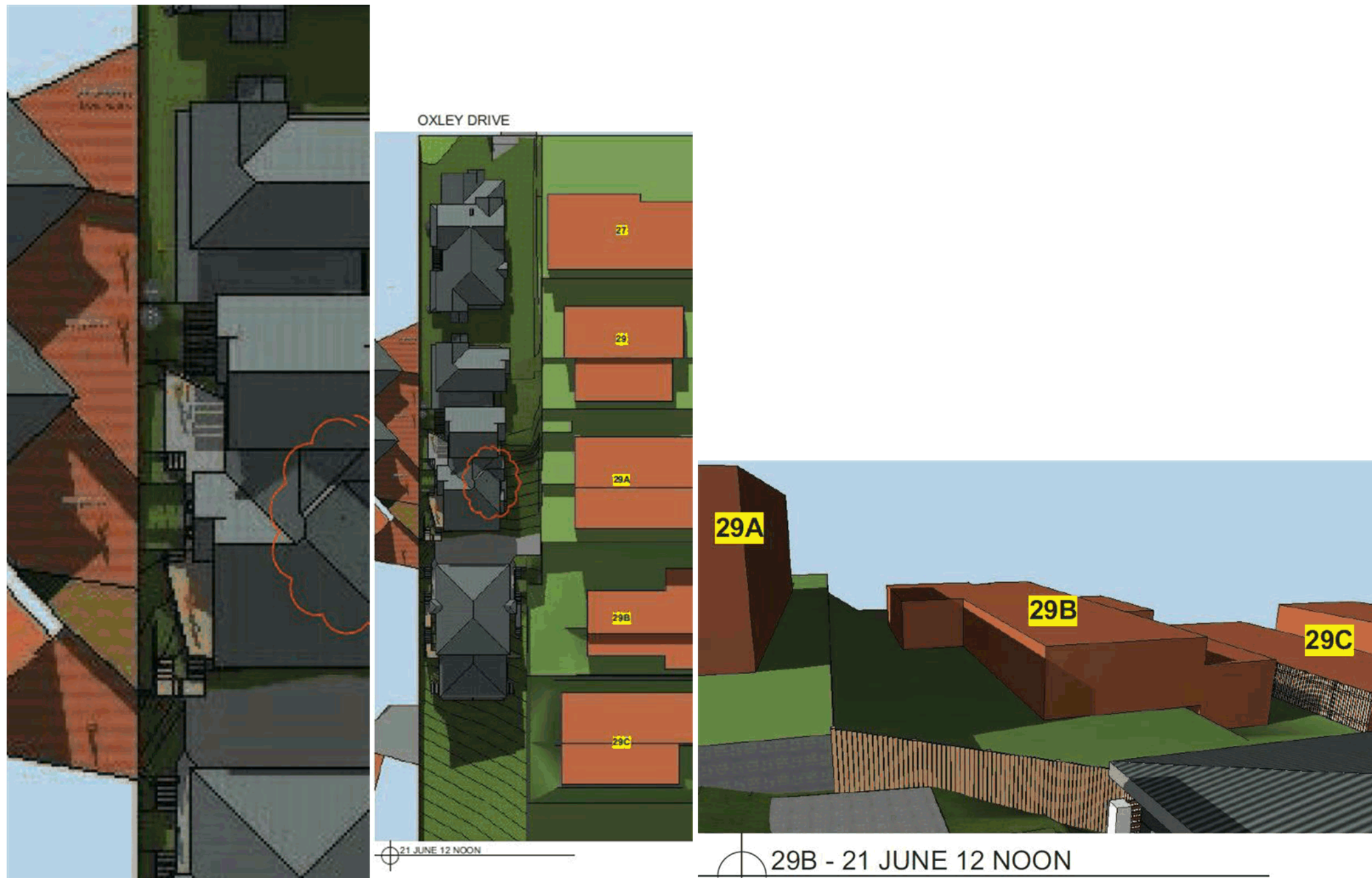
12 midday 21 June - Proposed development does not overshadow adjoining western units 3/23, 4/23, 5/23 and 6/23 private open space areas
