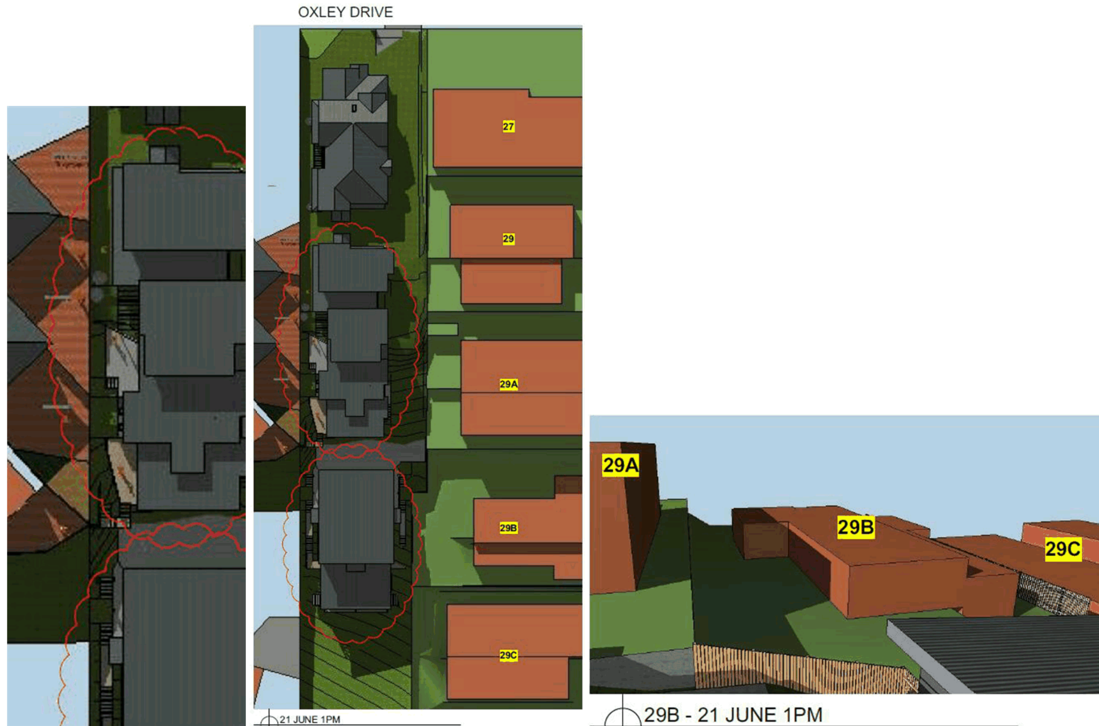
1:00pm 21 June - Proposed development does not overshadow adjoining western units 3/23, 4/23, 5/23 and 6/23 private open space areas Shadow impact upon 29B Oxley Drive cast from 29 A Oxley Drive and proposed development does not affect solar access to western facing living room window of 29B Oxley Drive.
