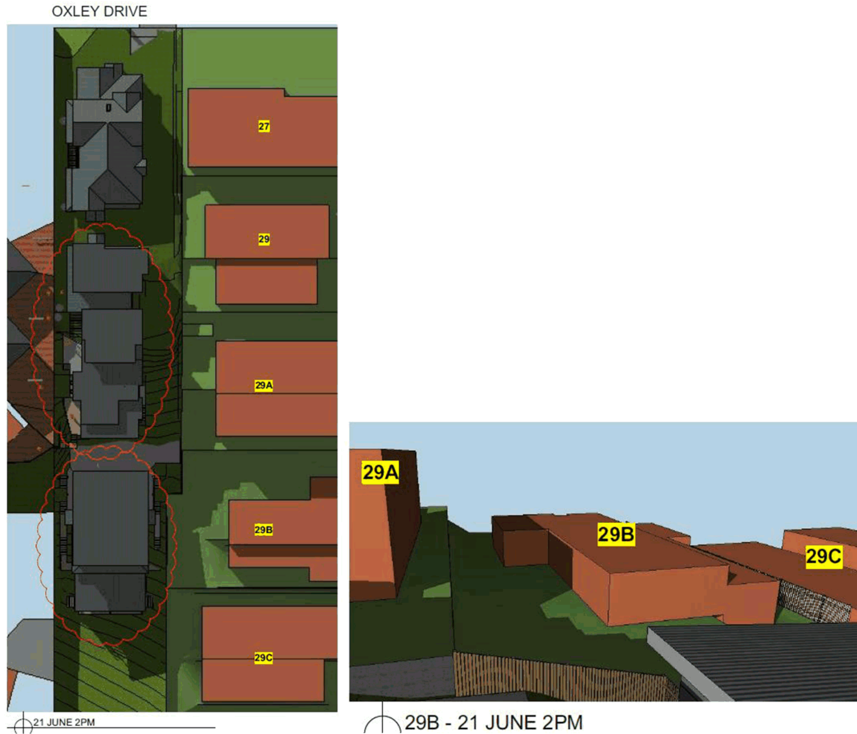
2:00 pm 21 June - Shadow impact upon 29B Oxley Drive cast from 29 A Oxley Drive and proposed development does not affect solar access to western facing living room window of 29B Oxley Drive.
