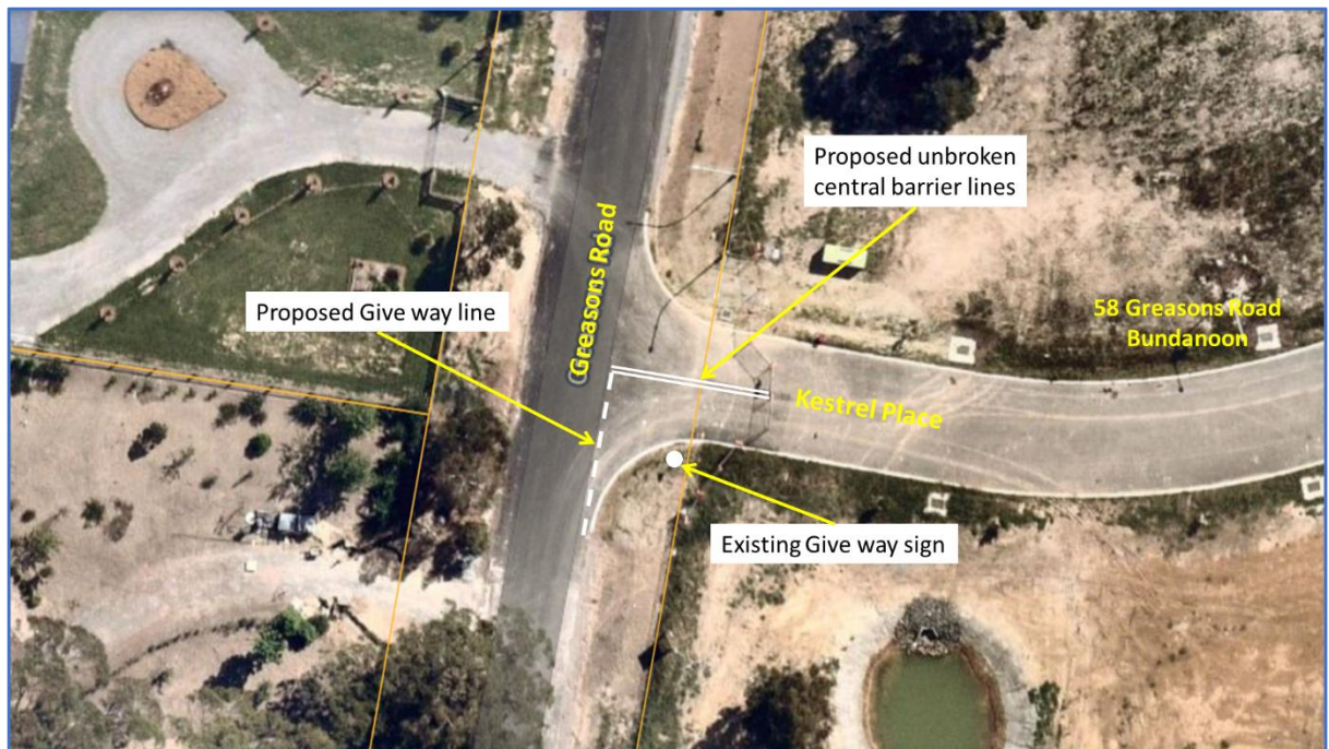
Fig.2- Intersection of Greasons Road and Kestrel Place
