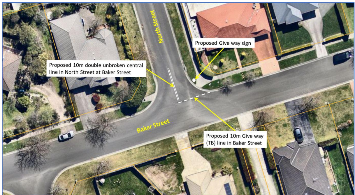
Fig.2- Plan showing proposed Give way restrictions in the intersection of North Street and Baker Street
