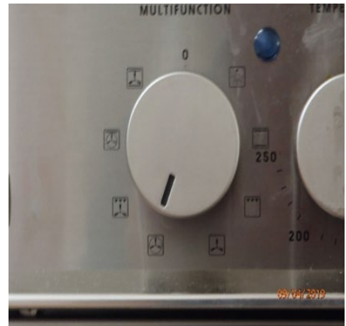
Figure 1: Multifunction oven switch.
